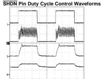
LM3501-16, 3 LEDs,  $R_{LED} = 22\Omega$ ,  $V_{IN} = 3.0V$ ,  $\overline{SHDN}$  frequency = 200 Hz
