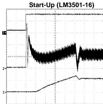
3 LEDs,  $R_{LED} = 22\Omega$ ,  $V_{IN} = 3.0V$ ,  $CNTRL = 2.7V$
