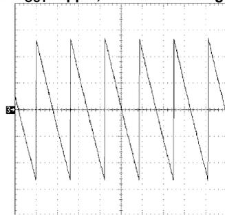
$V_{OUT}$  open circuit and equals approximately 15V DC,  $V_{IN} = 3.0V$
