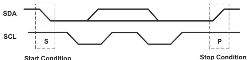
Figure 8-3. Definition of Start and Stop Conditions
