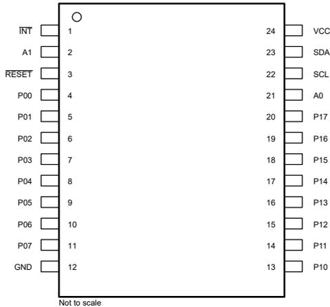
**Figure 5-1. PW (TSSOP) Package, 24-Pin (Top View)**
