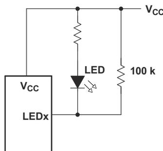
**Figure 9-2. High-Value Resistor in Parallel with LED**
