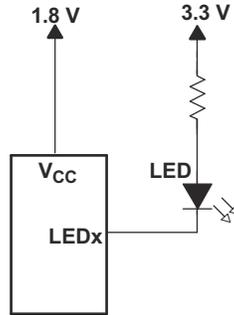
Figure 9-3. Device Supplied by a Lower Voltage
