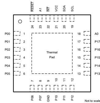
**Figure 5-2. RTW (WQFN) Package, 24-Pin (Top View)**
