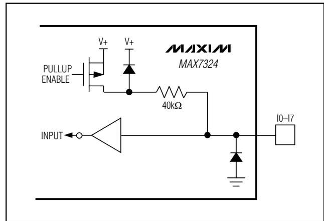
Figure 12. MAX7324 Input Port Structure
