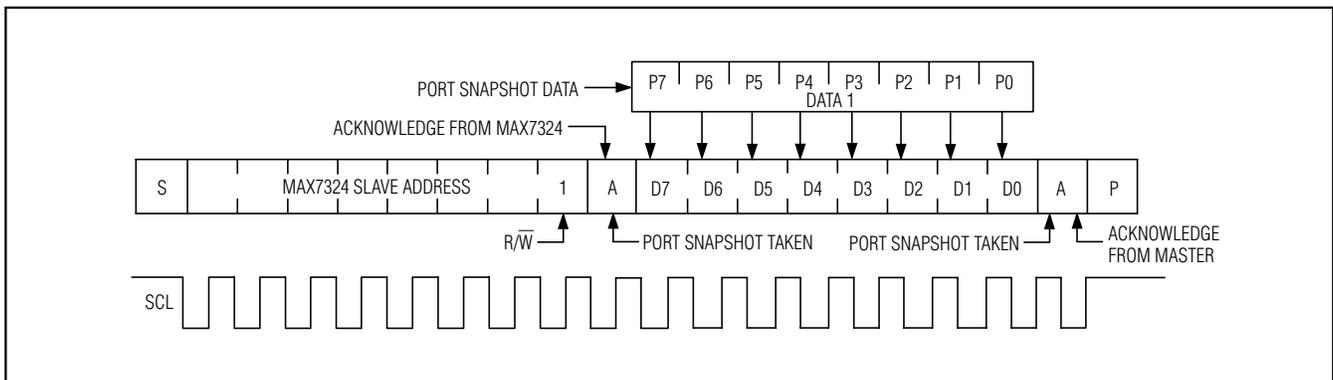
Figure 8. Reading Output Ports of the MAX7324
