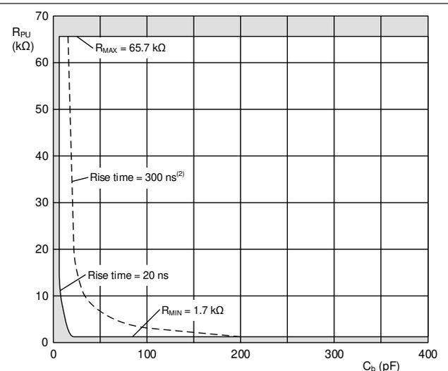
**Figure 8-5. Example Bus Requirements for 5 V Systems**
