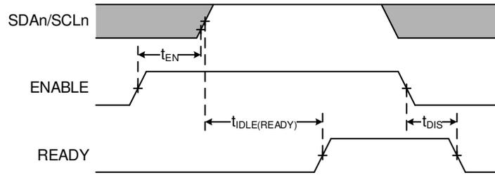
Figure 6-1. Timing for  $t_{EN}$ ,  $t_{IDLE(READY)}$ , and  $t_{DIS}$
