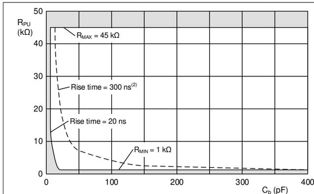
**Figure 8-4. Example Bus Requirements for 3.3 V Systems**
