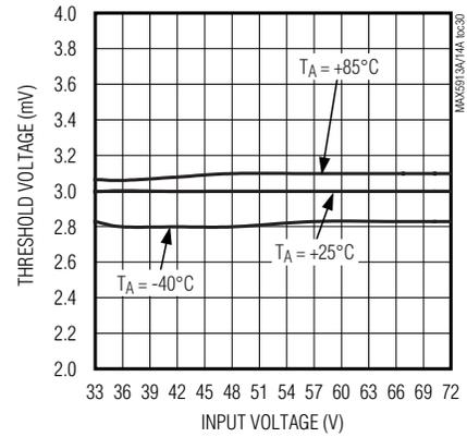
**OPEN-CIRCUIT THRESHOLD vs. TEMPERATURE**
