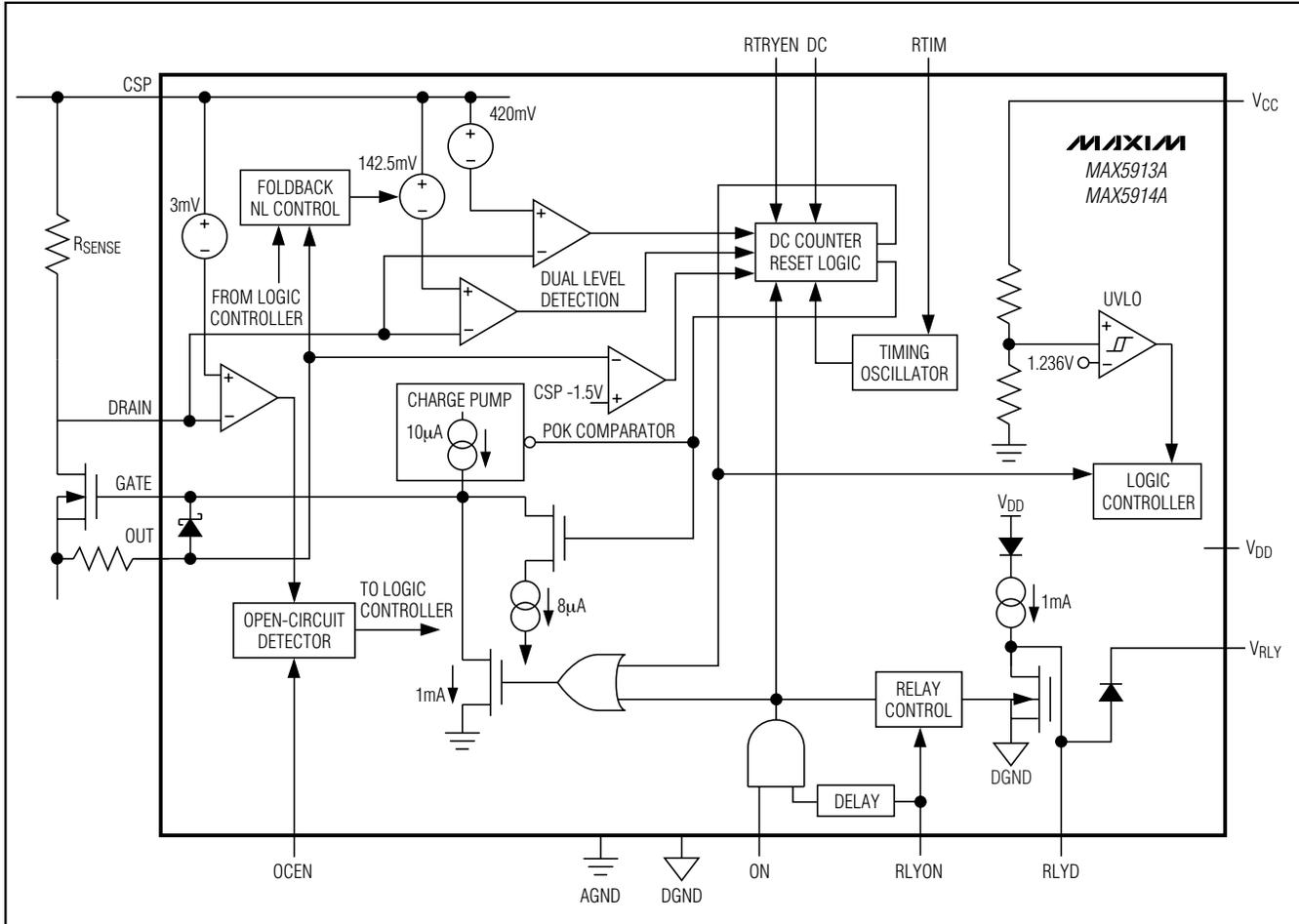
Figure 6. Functional Diagram
