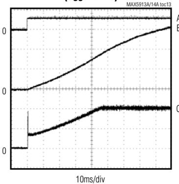
RLYON =  $V_{DD}$ ,  $R_L = 100\Omega$ ,  $R_{RTIM} = 40k\Omega$ ,  $C_{LOAD} = 470\mu F$
