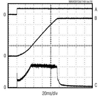
$RLYON = V_{DD}$ ,  $R_L = OPEN$ ,  $R_{RTIM} = 40k\Omega$ ,  $C_{LOAD} = 470\mu F$
