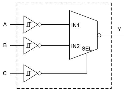
2 to 1 Data Selector with inverted output
