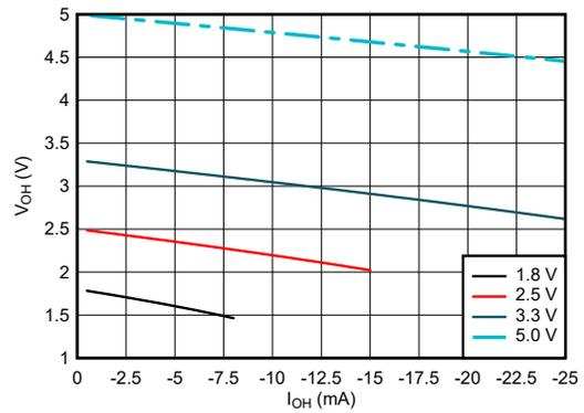
**Figure 5-4. Output Voltage vs Current in HIGH State**
