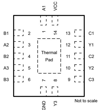
**Figure 4-2. SN74LVC3G98 BQA Package, 14-Pin WQFN (Top View)**
