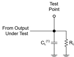
(1)  $C_L$  includes probe and test-fixture capacitance.
