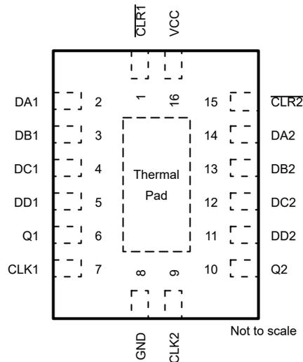
**Figure 4-1. BQB Package, 16-Pin WQFN (Top View)**
