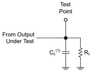
(1) C<sub>L</sub> includes probe and test-fixture capacitance.
