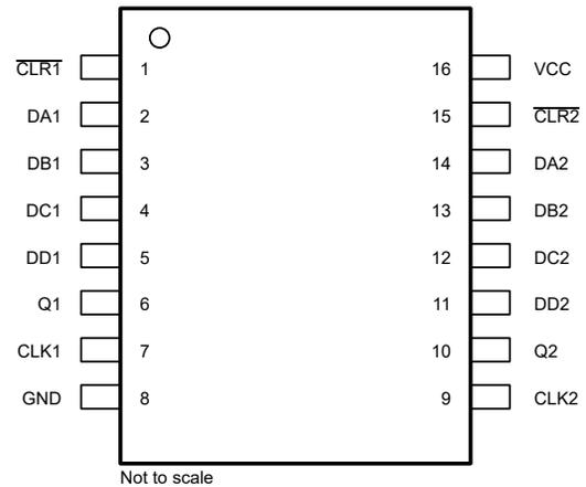
**Figure 4-2. PW Package, 16-Pin TSSOP (Preview) (Top View)**
