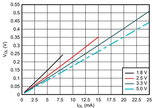
**Figure 5-5. Output Voltage vs Current in LOW State**
