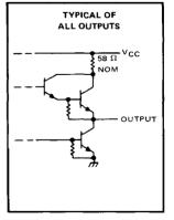
Not more than one output should be shorted at a time and duration of the short-circuit should not exceed 1 second.
