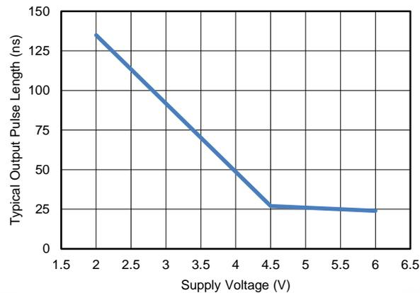
Figure 5. Typical Output Pulse Length Over V<sub>CC</sub> Range
