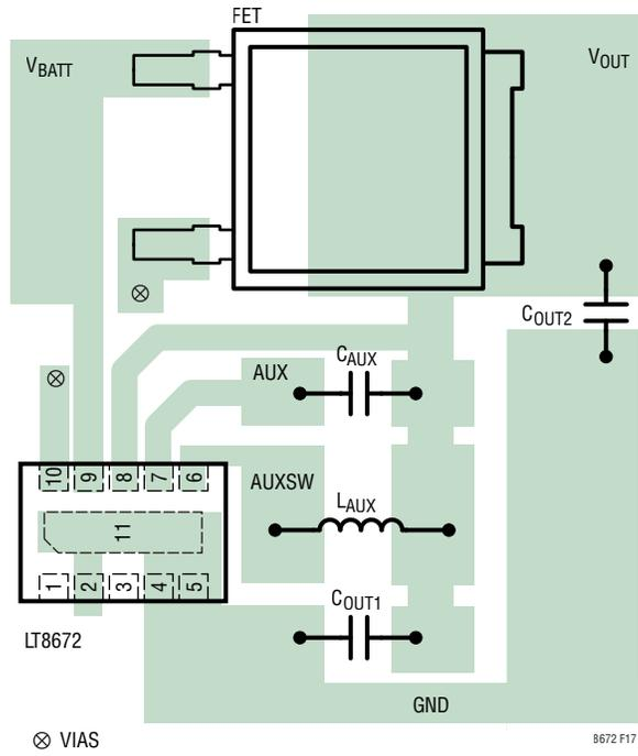
Figure 17. Recommended PCB Layout for the LT8672 (DFN)
