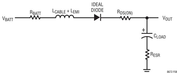
Figure 8. Simplified Application Model Including All Relevant Parasitics
