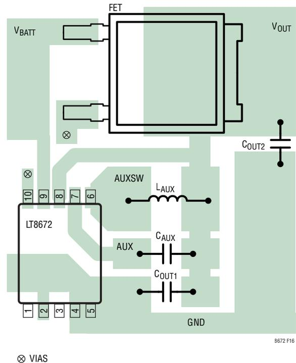
**Figure 16. Recommended PCB Layout for the LT8672 (MSOP)**
