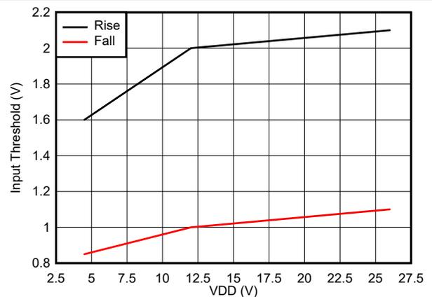
Figure 6-8. Input Thresholds
