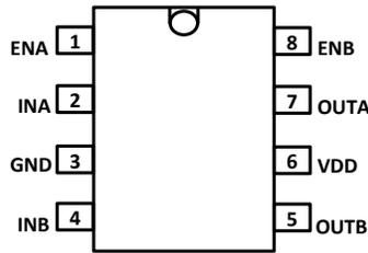
Figure 5-1. D Package 8-Pin SOIC Top View
