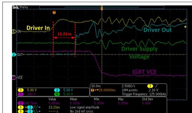
$V_{in} = 210\text{ V}$ ,  $V_{out} = 235\text{ V}$ ,  $I_{out} = 1.14\text{ A}$ ,  $F_{sw} = 125\text{ kHz}$ ,
