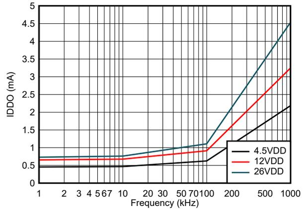
Figure 6-4. Operating Supply Current (Both Outputs Switching)
