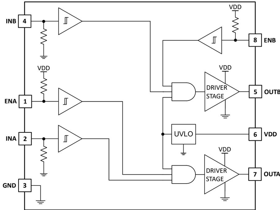
Typical ENx pullup resistance is 200 k $\Omega$  and INx pulldown resistance is 120 k $\Omega$ .
