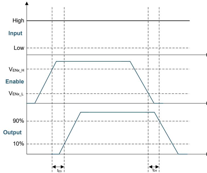
**Figure 6-1. Enable Function**
