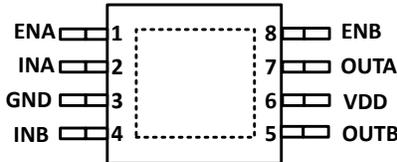
Figure 5-2. DGN Package 8-Pin VSSOP Top View
