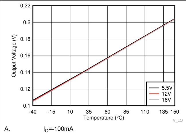
**Figure 6-14. LO High Output Voltage ( $V_{LOH}$ )**
