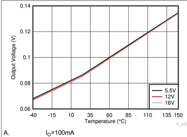
**Figure 6-13. LO Low Output Voltage ( $V_{LOL}$ )**
