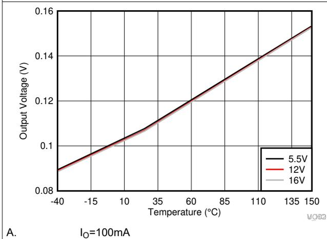
**Figure 6-15. HO Low Output Voltage ( $V_{HOL}$ )**
