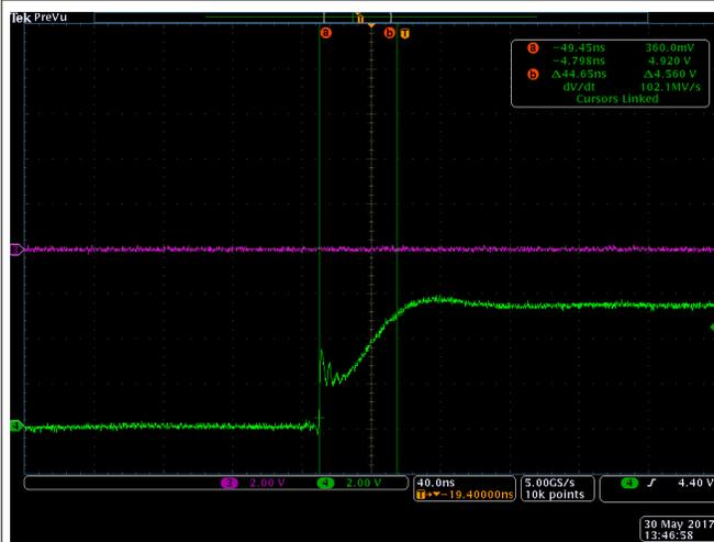
$V_{DD} = V_{HB} = 6\text{ V}$ , HS =  $C_{LOAD} = 10\text{ nF}$  Ch4 = HO
