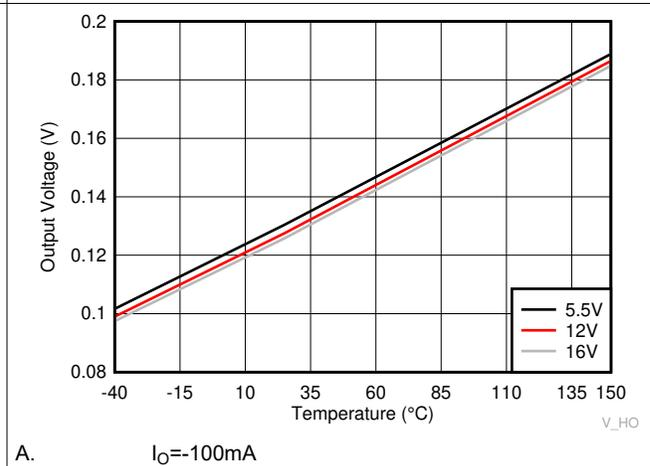
**Figure 6-16. HO High Output Voltage ( $V_{HOH}$ )**
