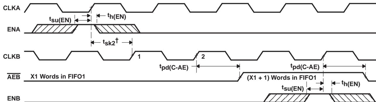
†  $t_{sk2}$  is the minimum time between a rising CLK<sub>A</sub> edge and a rising CLK<sub>B</sub> edge for  $\overline{AEB}$  to transition high in the next CLK<sub>B</sub> cycle. If the time between the rising CLK<sub>A</sub> edge and rising CLK<sub>B</sub> edge is less than  $t_{sk2}$ ,  $\overline{AEB}$  may transition high one CLK<sub>B</sub> cycle later than shown.
