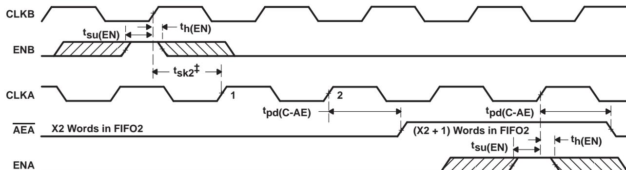
‡  $t_{sk2}$  is the minimum time between a rising CLK<sub>B</sub> edge and a rising CLK<sub>A</sub> edge for  $\overline{AEA}$  to transition high in the next CLK<sub>A</sub> cycle. If the time between the rising CLK<sub>B</sub> edge and rising CLK<sub>A</sub> edge is less than  $t_{sk2}$ ,  $\overline{AEA}$  may transition high one CLK<sub>A</sub> cycle later than shown.
