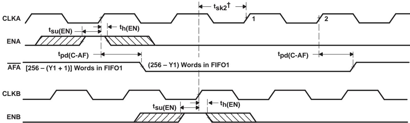
†  $t_{sk2}$  is the minimum time between a rising CLKA edge and a rising CLKB edge for  $\overline{AFA}$  to transition high in the next CLKA cycle. If the time between the rising CLKA edge and rising CLKB edge is less than  $t_{sk2}$ ,  $\overline{AFA}$  may transition high one CLKB cycle later than shown.
