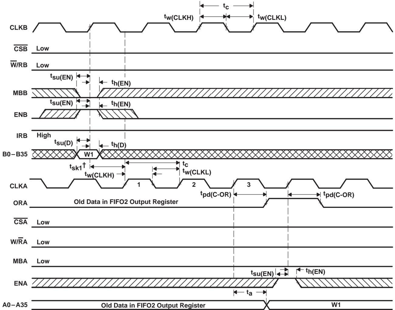
†  $t_{sk1}$  is the minimum time between a rising CLKB edge and a rising CLKA edge for ORA to transition high and to clock the next word to the FIFO2 output register in three CLKA cycles. If the time between the rising CLKB edge and rising CLKA edge is less than  $t_{sk1}$ , the transition of ORA high and load of the first word to the output register may occur one CLKA cycle later than shown.
