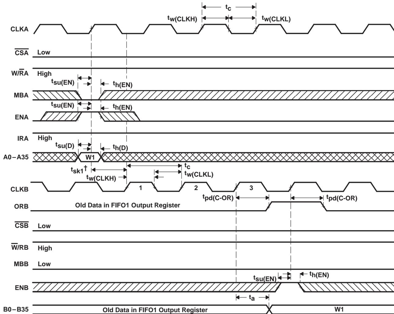
†  $t_{sk1}$  is the minimum time between a rising CLKA edge and a rising CLKB edge for ORB to transition high and to clock the next word to the FIFO1 output register in three CLKB cycles. If the time between the rising CLKA edge and rising CLKB edge is less than  $t_{sk1}$ , the transition of ORB high and load of the first word to the output register may occur one CLKB cycle later than shown.
