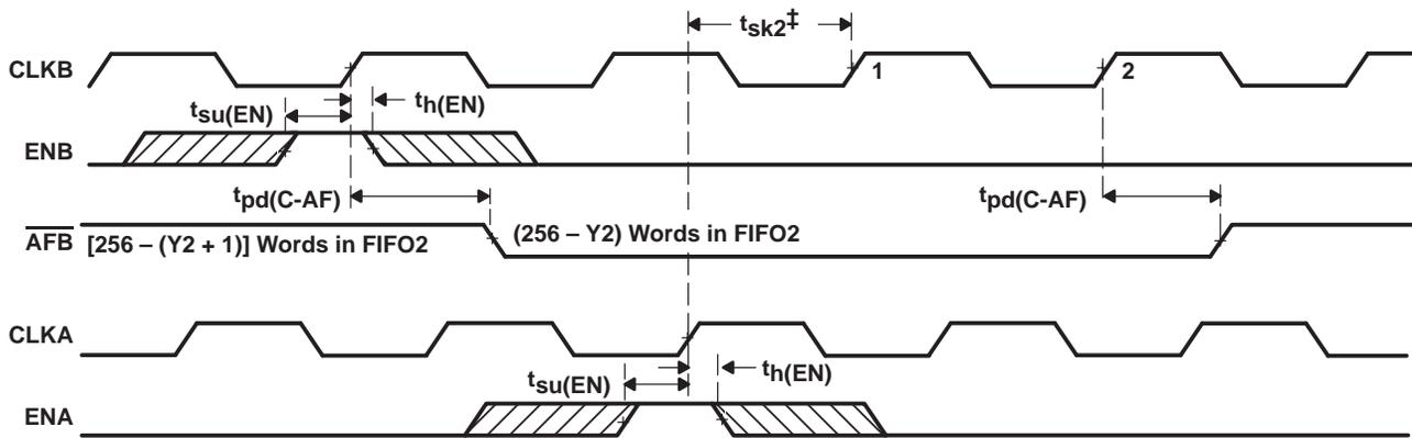
‡  $t_{sk2}$  is the minimum time between a rising CLKB edge and a rising CLKA edge for  $\overline{AFB}$  to transition high in the next CLKB cycle. If the time between the rising CLKB edge and rising CLKA edge is less than  $t_{sk2}$ ,  $\overline{AFB}$  may transition high one CLKA cycle later than shown.
