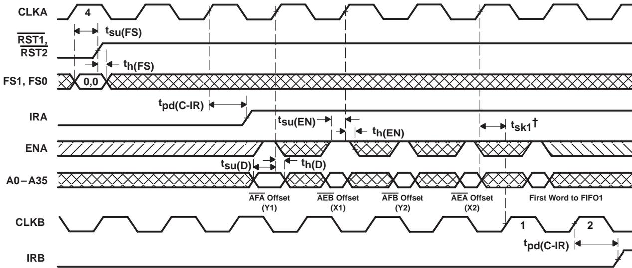
†  $t_{sk1}$  is the minimum time between the rising CLKA edge and a rising CLKB edge for IRB to transition high in the next cycle. If the time between the rising edge of CLKA and rising edge of CLKB is less than  $t_{sk1}$ , IRB may transition high one cycle later than shown.
