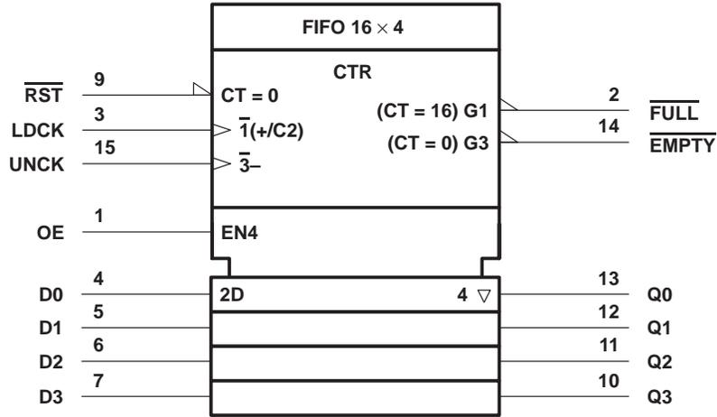
† This symbol is in accordance with ANSI/IEEE Standard 91-1984 and IEC Publication 617-12. The symbol is functionally accurate but does not show the details of implementation; for these, see the logic diagram. The symbol represents the memory as if it were controlled by a single counter whose content is the number of words stored at the time. Output data is invalid when the counter content (CT) is 0. Pin numbers shown are for the DW and N packages.
