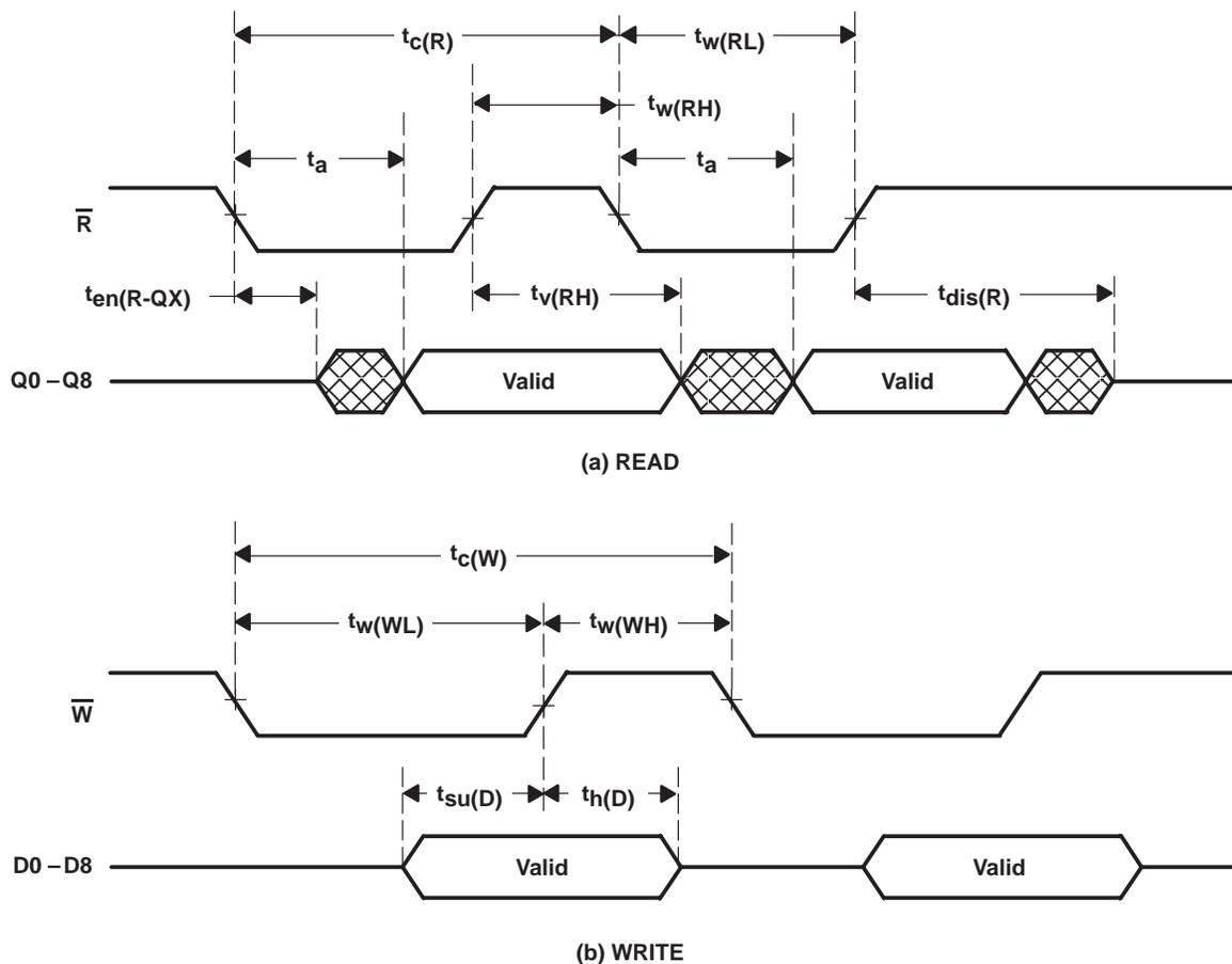
Figure 1. Asynchronous Waveforms
