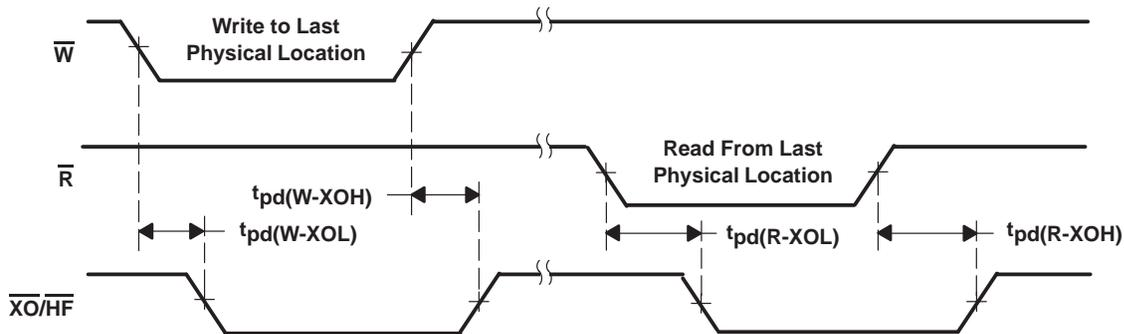
Figure 9. Expansion-Out Waveforms
