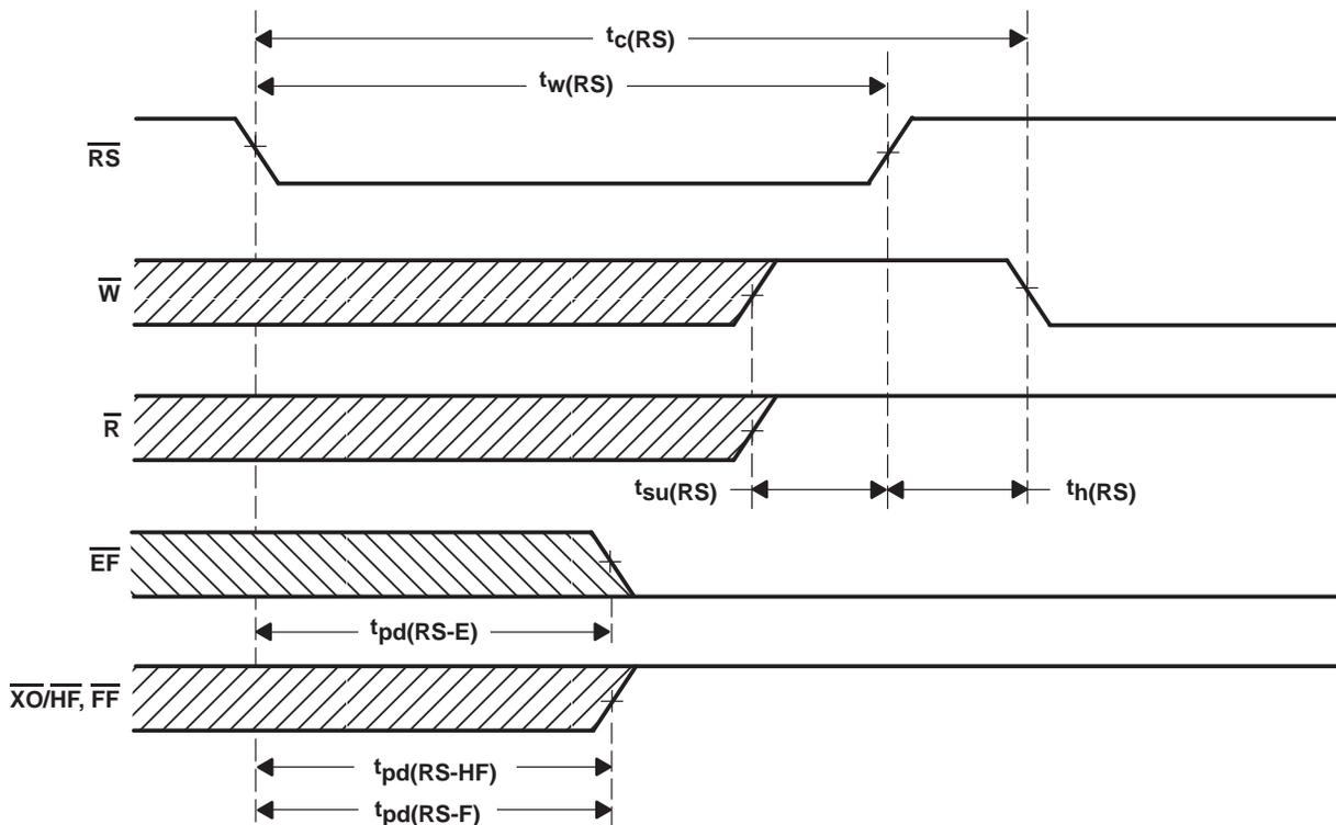
Figure 7. Master-Reset Waveforms
