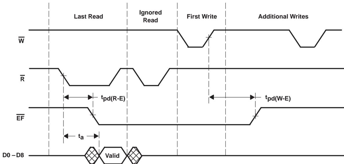
Figure 3. Empty-Flag Waveforms
