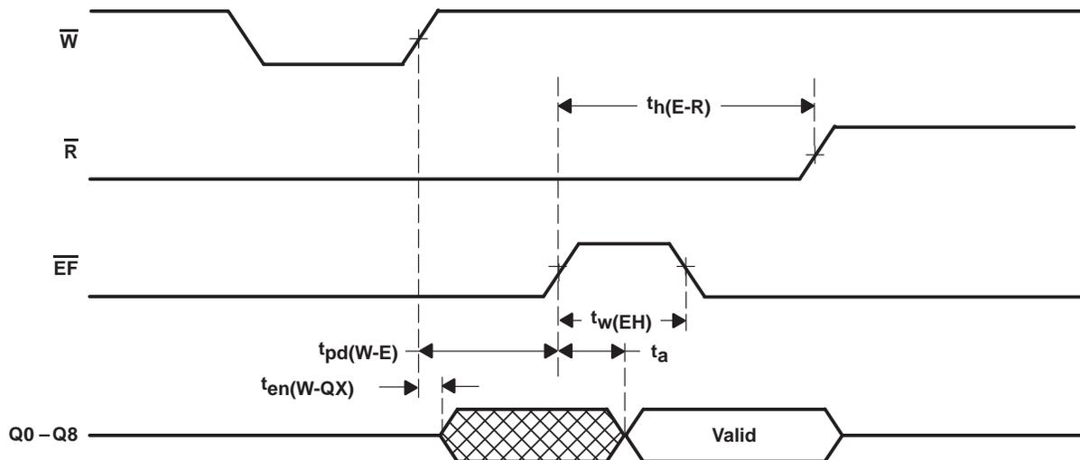
Figure 5. Automatic-Read Waveforms
