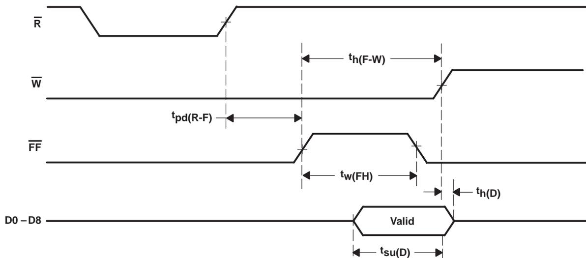
Figure 6. Automatic-Write Waveforms
