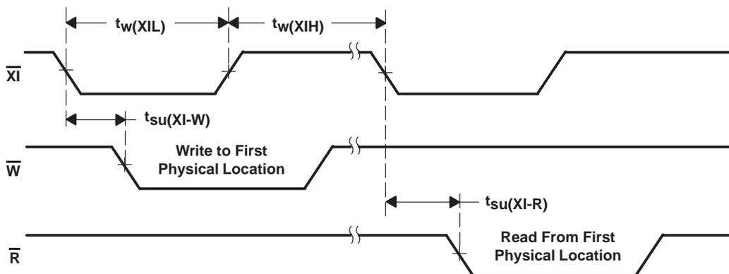
Figure 10. Expansion-In Waveforms
