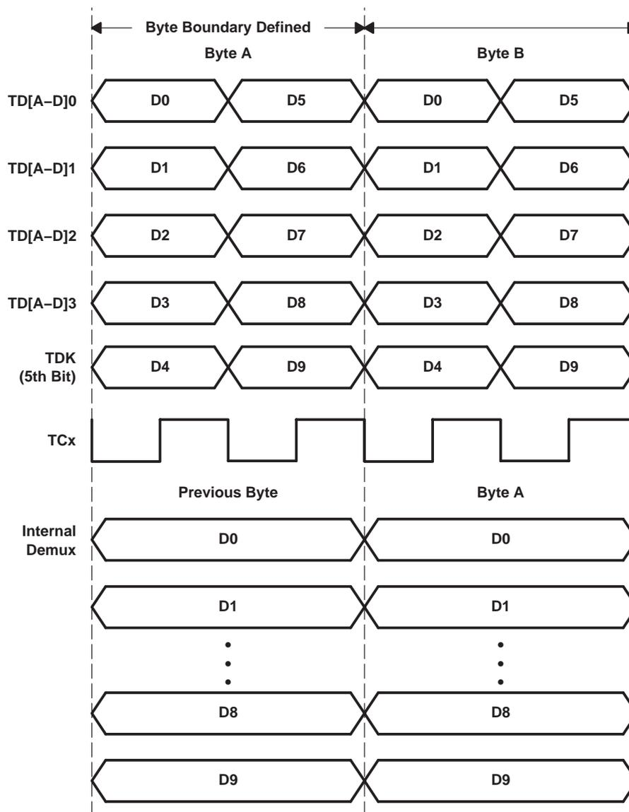
**Figure 16. Transmit Data Mapping Under 8-b/10-b Bypass**
