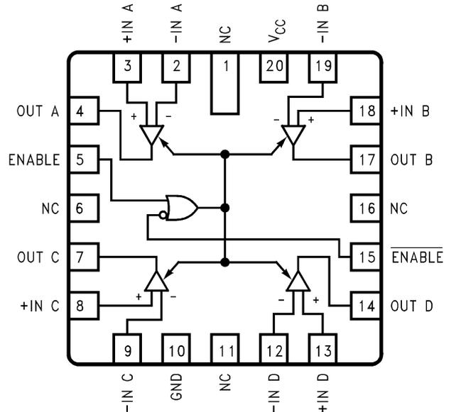
Figure 2. 20-Lead LCCC Package-Top View
