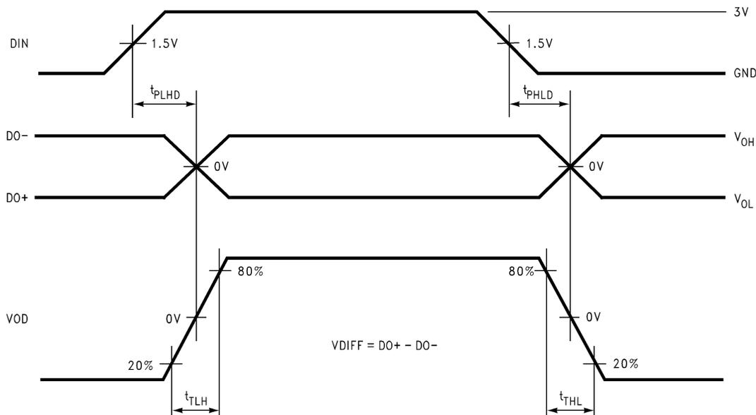
Generator waveform for all tests unless otherwise specified:  $f = 1 \text{ MHz}$ , Duty Cycle = 50%,  $Z_o = 50\Omega$ ,  $t_r \leq 10 \text{ ns}$ ,  $t_f \leq 10 \text{ ns}$ .
