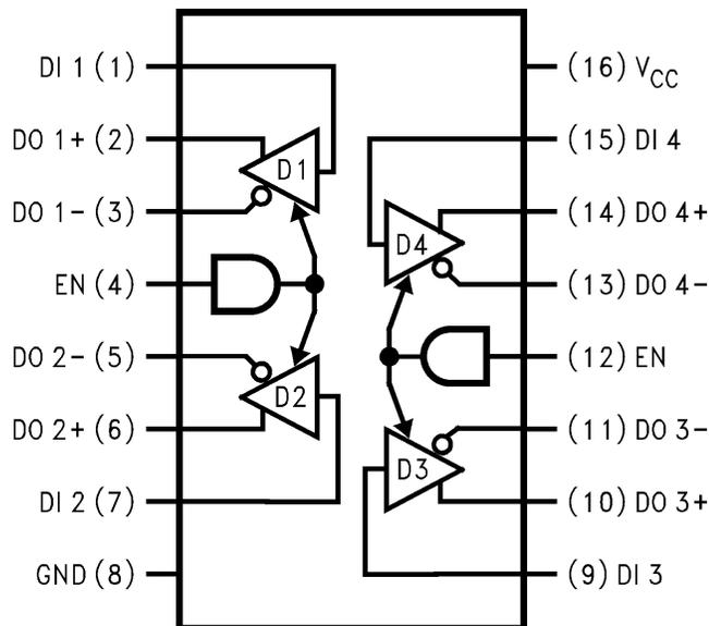
**Figure 1. Dual-In-Line Package (Top View)**
