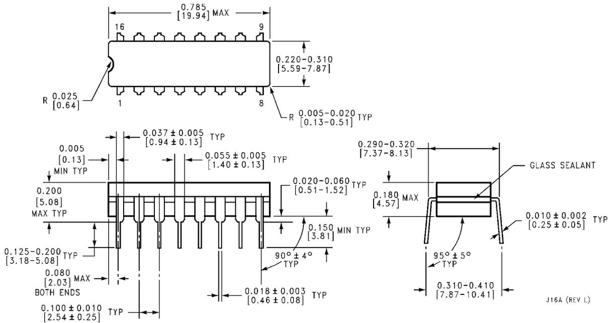
**16-Lead Ceramic Dual-In-Line Package (J)**
