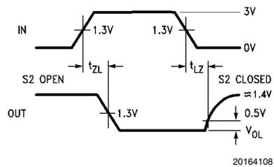
**Note 9:** The input pulse is supplied by a generator having the following characteristics:  $f = 1.0 \text{ MHz}$ , 50% duty cycle,  $t_r \leq 6.0 \text{ ns}$ ,  $t_f \leq 6.0 \text{ ns}$ ,  $Z_0 = 50\Omega$ .
