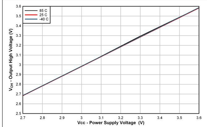
Figure 3. Output High Voltage vs Power Supply Voltage
