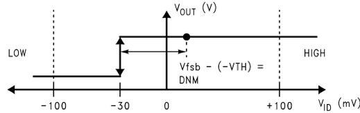
**Figure 11. VTC of the DS90LT012AH LVDS Receiver**
