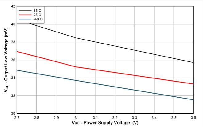
Figure 4. Output Low Voltage vs Power Supply Voltage
