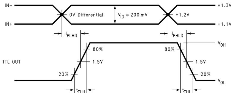
Figure 10. Receiver Propagation Delay and Transition Time Waveforms
