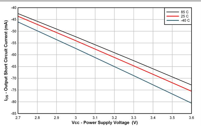
Figure 2. Output Short-Circuit Current vs Power Supply Voltage
