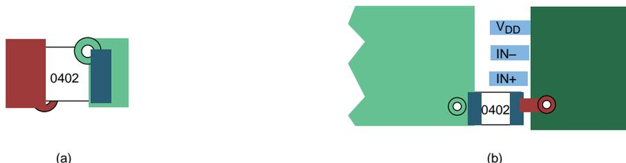
Figure 22. Typical Decoupling Capacitor Layouts
