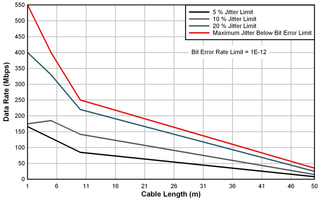
Figure 15. DS90LT012AH Performance: Cable Length vs Data Rate
