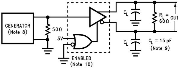
FIGURE 3. Differential Output Delay and Transition Times
