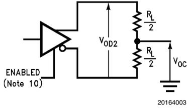
FIGURE 1. Differential and Common Mode Output Voltage
