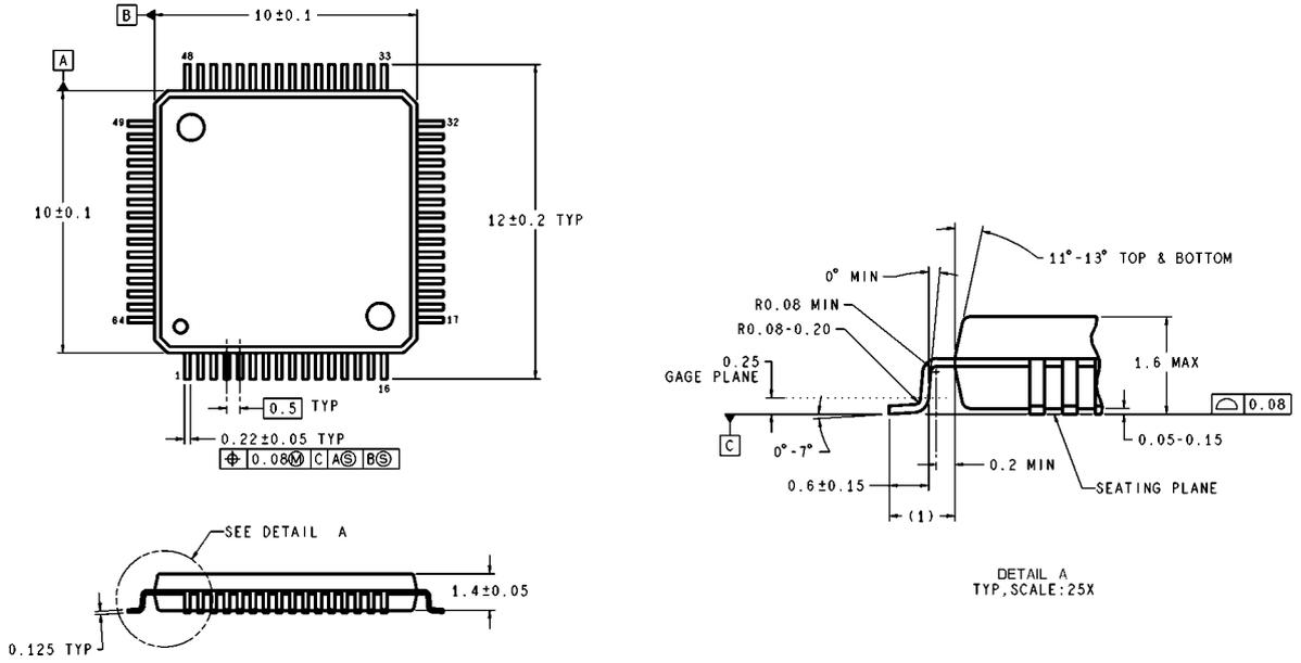
DIMENSIONS ARE IN MILLIMETERS
