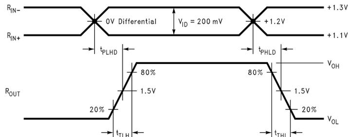
Figure 5. Receiver Propagation Delay and Transition Time Waveforms
