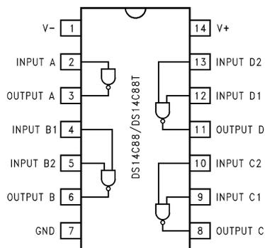
**Figure 1. SOIC or PDIP Package- Top View
