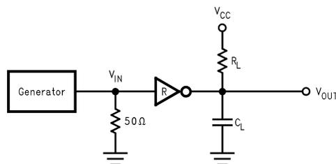
Generator characteristics for receiver input:  $f = 64\text{ kHz}$  ( $128\text{ kbits/sec}$ ),  $t_r = t_f = 200\text{ ns}$ ,  $V_{IH} = 3\text{V}$ ,  $V_{IL} = -3\text{V}$ , duty cycle = 50%.
