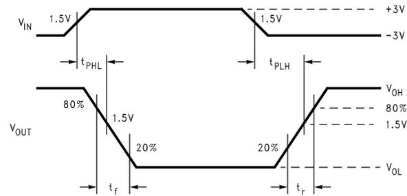
**Figure 6. Receiver Propagation Delay and Transition Time Waveform**
