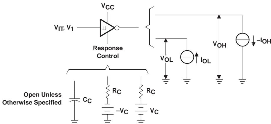
NOTE A: Arrows indicate actual direction of current flow. Current into a terminal is a positive value.
