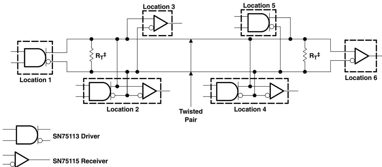
†  $R_T = Z_0$ . A capacitor may be connected in series with  $R_T$  to reduce power dissipation.
