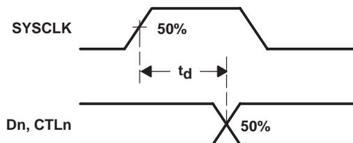
Figure 2. Dn and CTLn Output-Delay Timing Waveforms
