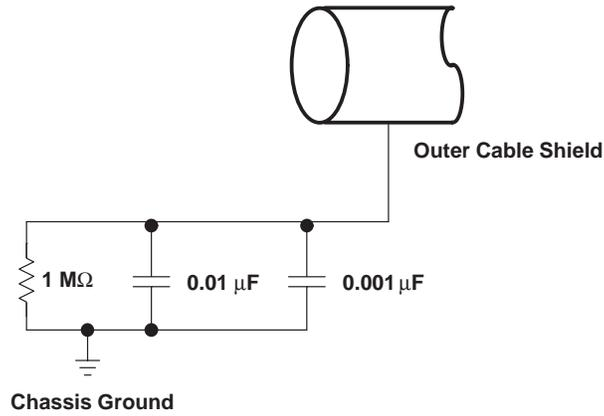
Figure 5. Compliant DC Isolated Outer Shield Termination
