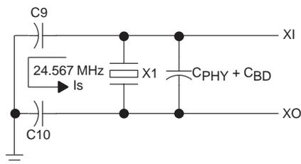
**Figure 9. Load Capacitance for the TSB21LV03C PHY**
