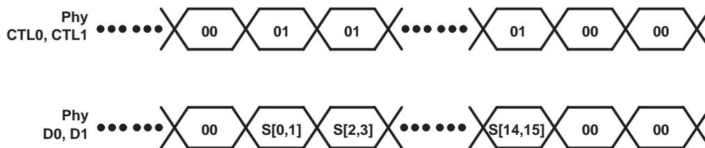
**Figure 12. Status Transfer Timing**
