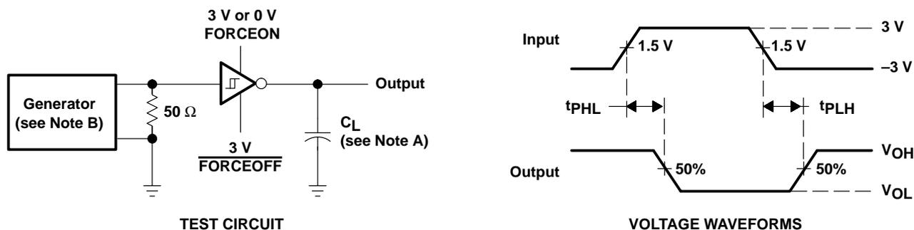
NOTES: C.  $C_L$  includes probe and jig capacitance.
