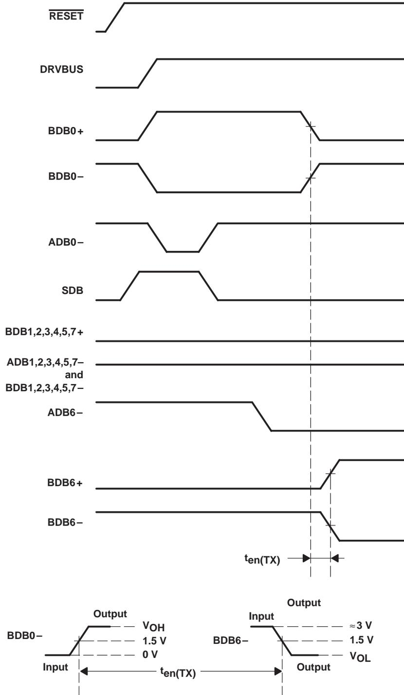
Figure 7. Receive-to-Transmit ( $t_{en(TX)}$ ) Timing Waveforms
