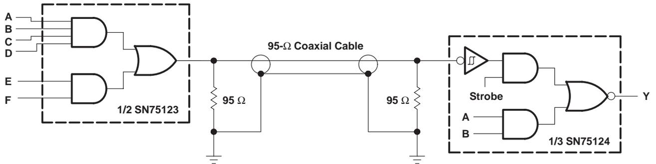
Figure 3. Unbalanced Line Communication Using SN75123 and SN75124
