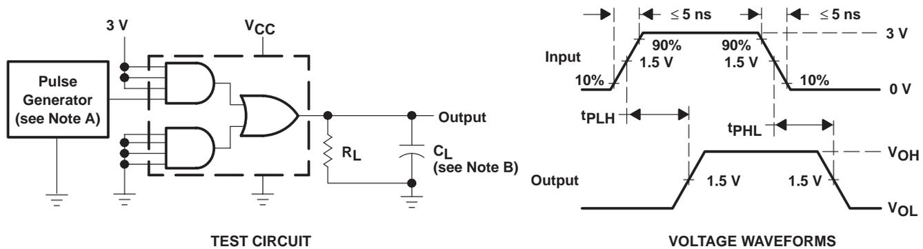
NOTES: A. The pulse generator has the following characteristics:  $Z_O \approx 50\ \Omega$ ,  $t_w = 200\text{ ns}$ , duty cycle  $\leq 50\%$ , PRR  $\leq 500\text{ kHz}$ .
