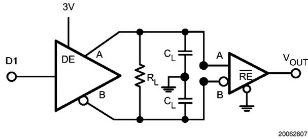
FIGURE 5. Test Circuit for Receiver Propagation Delay
