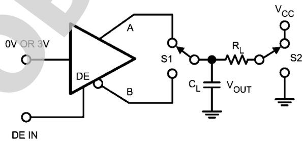
FIGURE 4. Test Circuit for Driver Enable / Disable
