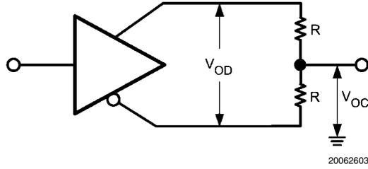
FIGURE 1. Test Circuit for  $V_{OD}$  and  $V_{OC}$
