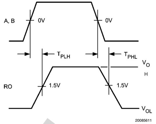
FIGURE 9. Receiver Propagation Delay
