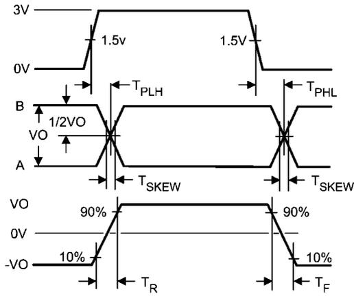
FIGURE 7. Driver Propagation Delay, Rise / Fall Time
