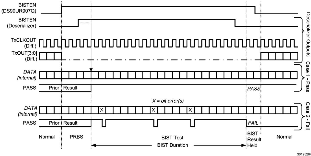
FIGURE 26. BIST Waveforms
