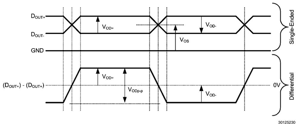
FIGURE 3. Channel Link II Single-ended and Differential Waveforms
