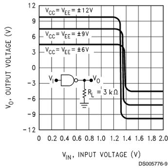
**FIGURE 1. Transfer Characteristics vs Power Supply Voltage**
