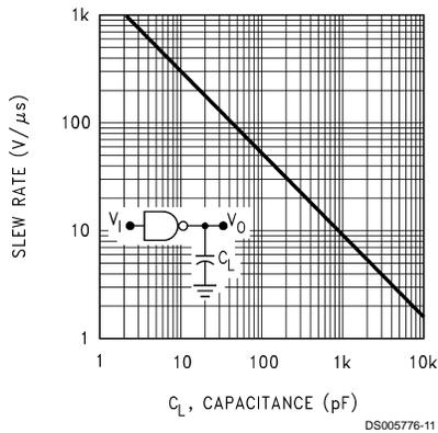
**FIGURE 3. Output Slew Rate vs Load Capacitance**
