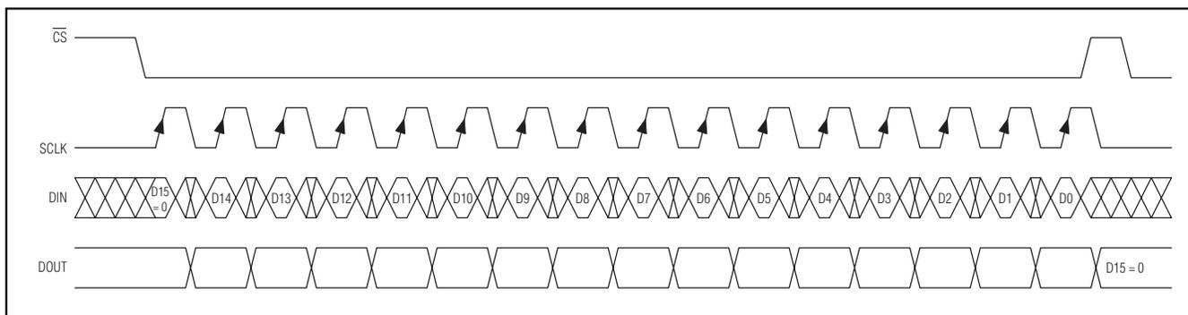
Figure 5. 16-Bit Write Transmission to the MAX6957
