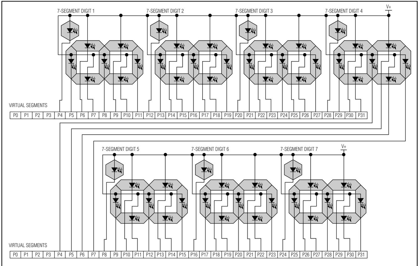
Figure 2. Two MAX6957s Controlling Seven 7-Segment Displays
