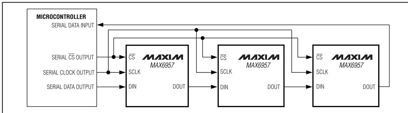
Figure 4. Daisy-Chain Arrangement for Controlling Multiple MAX6957s
