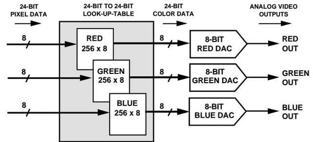
Figure 18. 24-Bit to 24-Bit Direct True-Color Configuration
