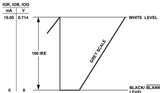
Figure 31. Composite Video Waveform (Pedestal = 0 IRE;  $R_{SET} = 259 \Omega$ )
