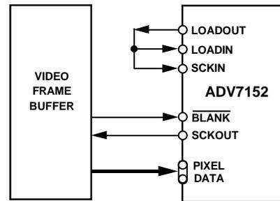
Figure 16. ADV7152 Interface Using SCKIN and SCKOUT
