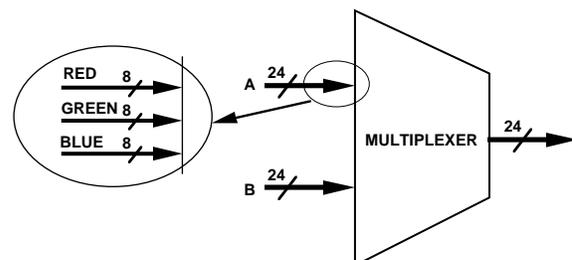
Figure 10. Multiplexed Color Inputs for the ADV7152
