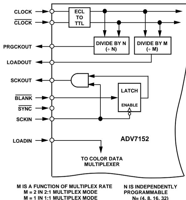
Figure 12. Clock Control Circuit of the ADV7152
