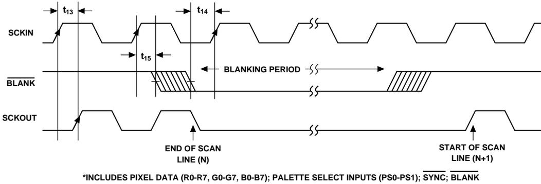
Figure 7. Video Data Shift Clock Input (SCKIN) & BLANK vs. Video Data Shift Clock Output (SCKOUT)
