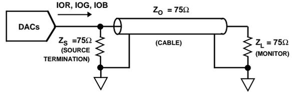
Figure 27. DAC Output Termination (Doubly Terminated  $75 \Omega$  Load)
