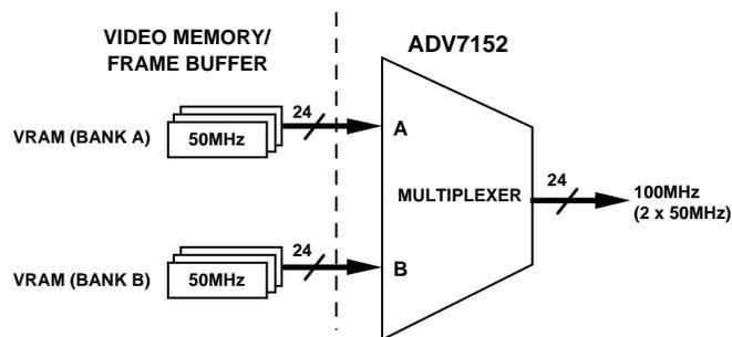
Figure 11. Direct Interfacing of Video Memory to ADV7152
