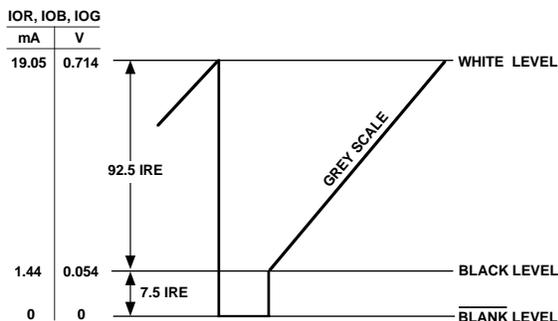
Figure 30. Composite Video Waveform (Pedestal = 7.5 IRE;  $R_{SET} = 280 \Omega$ )
