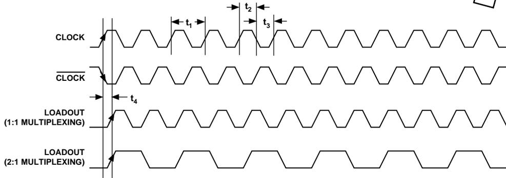
Figure 2. LOADOUT vs. Pixel Clock Input (CLOCK,  $\overline{\text{CLOCK}}$ )
