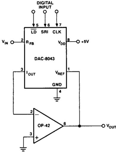
Figure 8. Analog/Digital Divider
