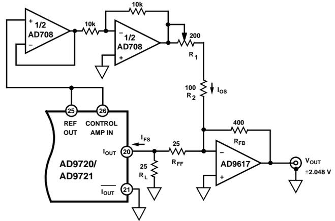
Figure 3. I/V Conversion Using Current Feedback Amp
