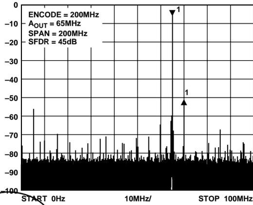
Figure 14. Wideband SFDR 65 MHz  $A_{OUT}$ ; 200 MHz Clock
