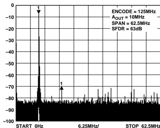
Figure 10. Wideband SFDR 10 MHz  $A_{OUT}$ ; 125 MHz Clock
