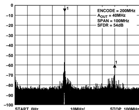
Figure 13. Wideband SFDR 40 MHz  $A_{OUT}$ ; 200 MHz Clock
