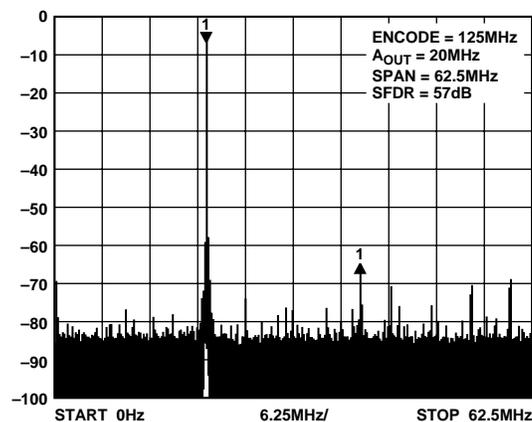
Figure 11. Wideband SFDR 20 MHz  $A_{OUT}$ ; 125 MHz Clock
