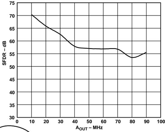
Figure 2. Narrowband SFDR (Clock = 200 MHz) vs.  $A_{OUT}$  Frequency
