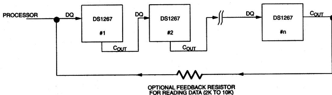
The  $C_{OUT}$  output of the DS1267 can be used to drive the DQ input of another DS1267. When connecting multiple devices, the total number of bits transmitted is always 17 times the number of DS1267s in the daisy chain.
