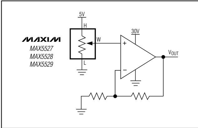
Figure 7. Positive LCD Bias Control Using a Voltage-Divider
