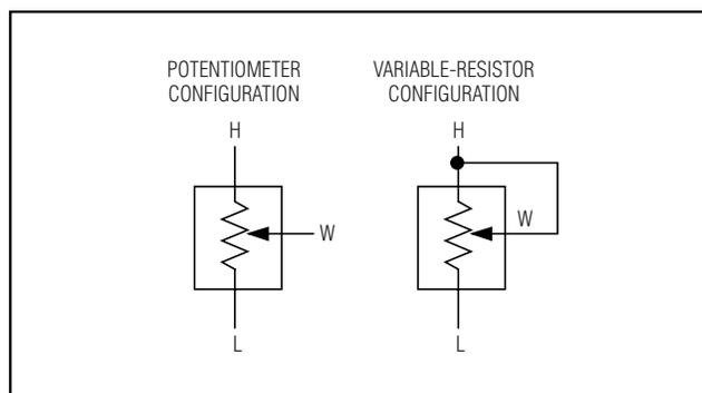
Figure 1. Potentiometer/Variable-Resistor Configuration
