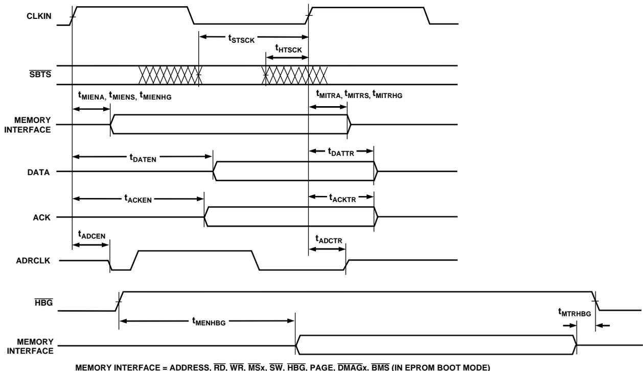
MEMORY INTERFACE = ADDRESS,  $\overline{\text{RD}}$ ,  $\overline{\text{WR}}$ ,  $\overline{\text{MSx}}$ ,  $\overline{\text{SW}}$ ,  $\overline{\text{HBG}}$ , PAGE,  $\overline{\text{DMAGx}}$ , BMS (IN EPROM BOOT MODE)
