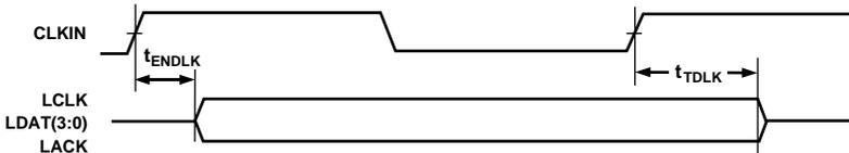
LINK PORT ENABLE OR THREE-STATE TAKES EFFECT 2 CYCLES AFTER A WRITE TO A LINK PORT CONTROL REGISTER.
