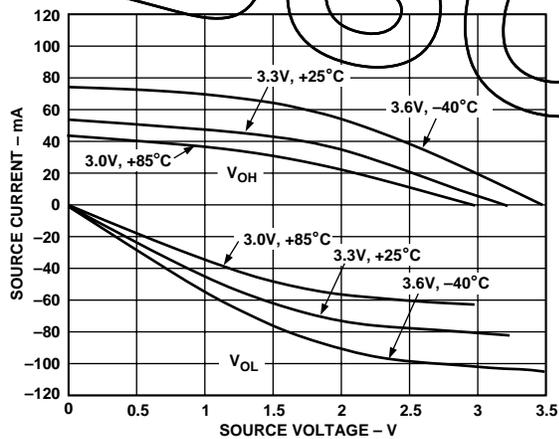
Figure 27. ADSP-2106x Typical Drive Currents ( $V_{DD} = 3.3 V$ )
