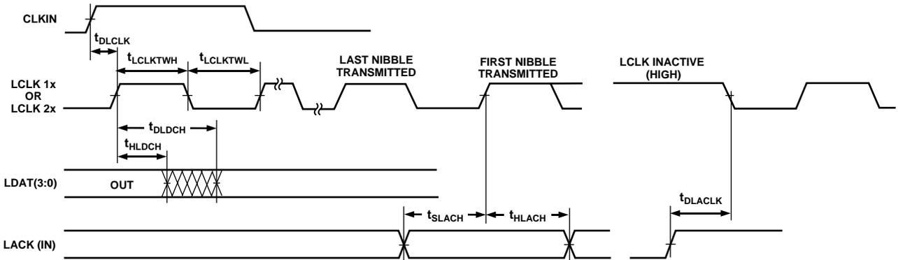
THE  $t_{SLACH}$  REQUIREMENT APPLIES TO THE RISING EDGE OF LCLK ONLY FOR THE FIRST NIBBLE TRANSMITTED.
