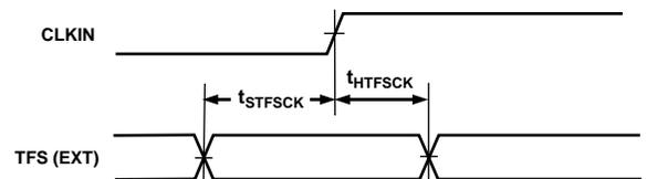
NOTE: APPLIES ONLY TO GATED SERIAL CLOCK MODE WITH EXTERNAL TFS, AS USED IN THE SERIAL PORT SYSTEM I/O FOR MESH MULTIPROCESSING.
