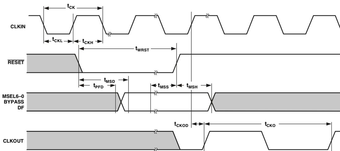
Figure 6. Clock In and Clock Out Cycle Timing
