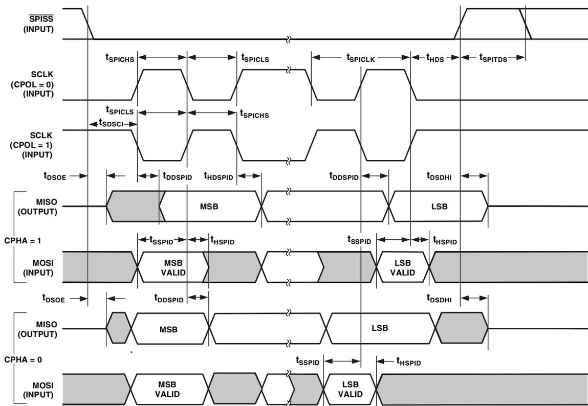
Figure 16. Serial Peripheral Interface (SPI) Port—Slave Timing
