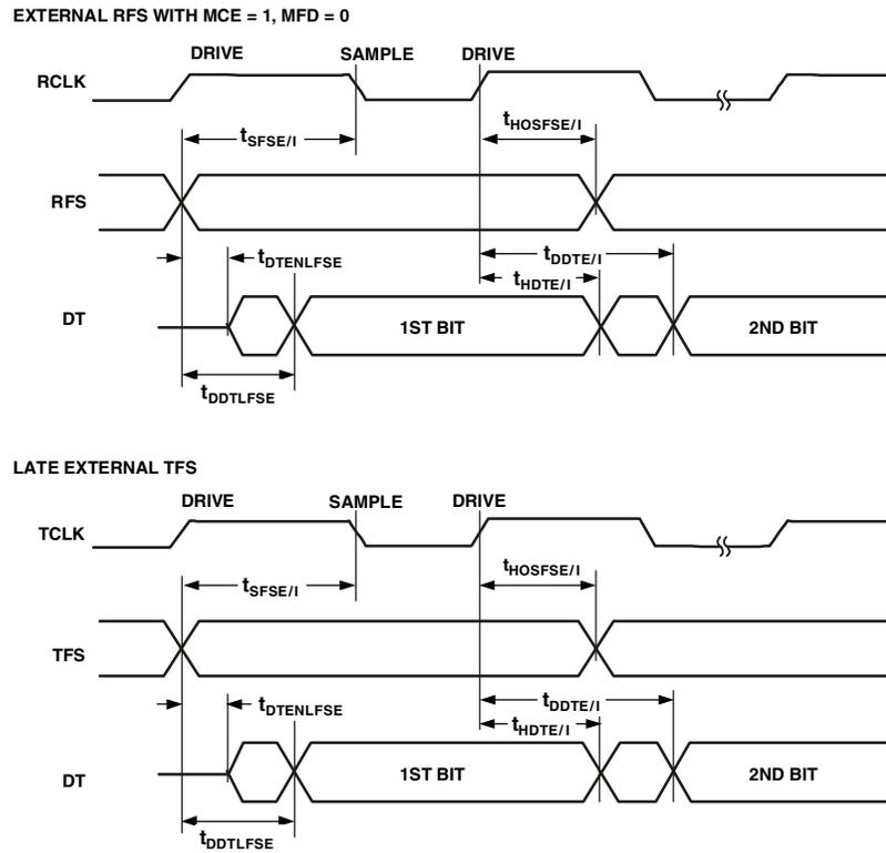
Figure 13. Serial Port—External Late Frame Sync (Frame Sync Setup > 0.5t<sub>SCLK</sub>)
