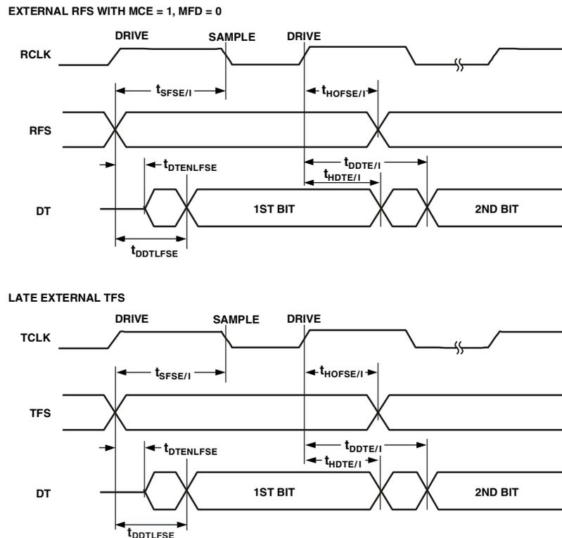
Figure 14. Serial Port—External Late Frame Sync (Frame Sync Setup < 0.5t<sub>HCLK</sub>)
