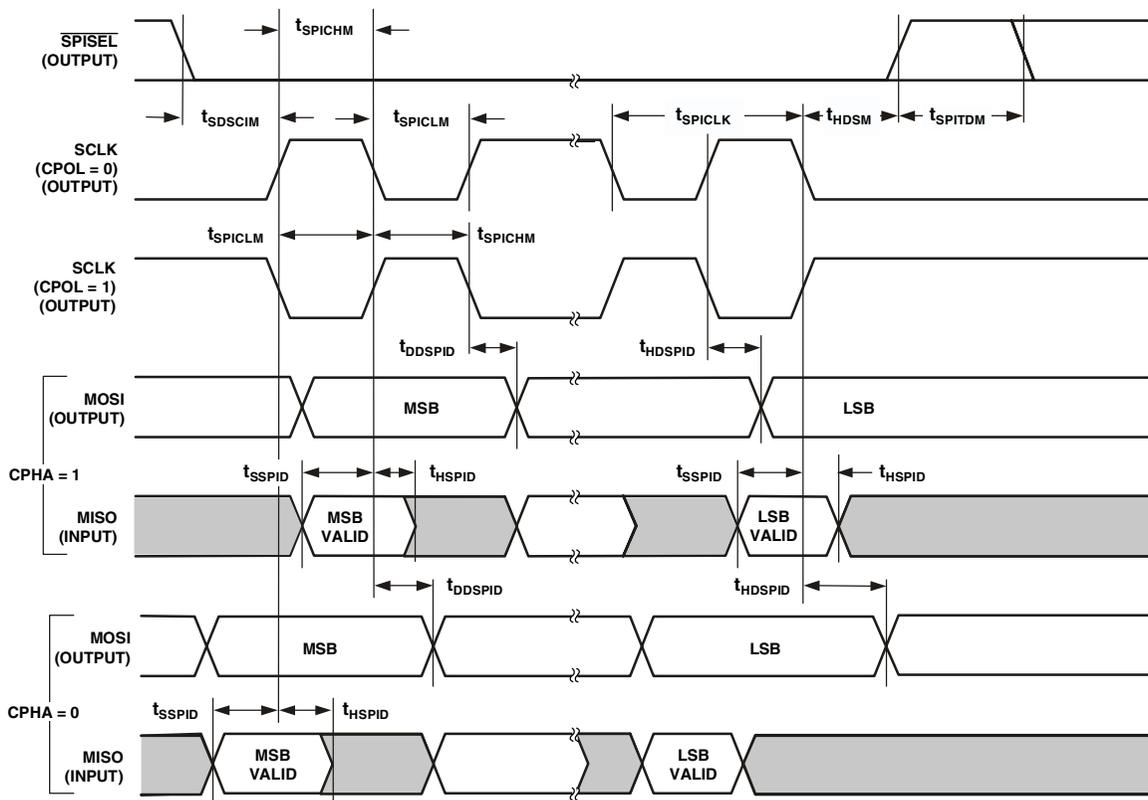
Figure 15. Serial Peripheral Interface (SPI) Port—Master Timing
