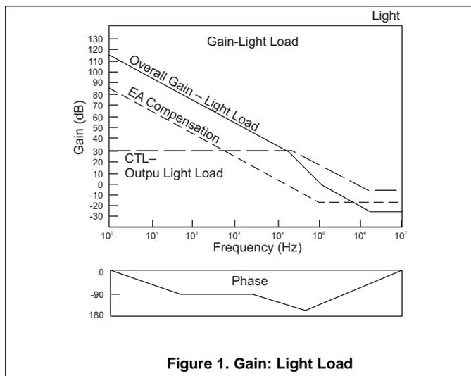
Figure 1. Gain: Light Load
