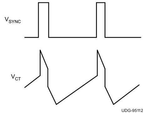
Figure 10. Operational Waveforms
