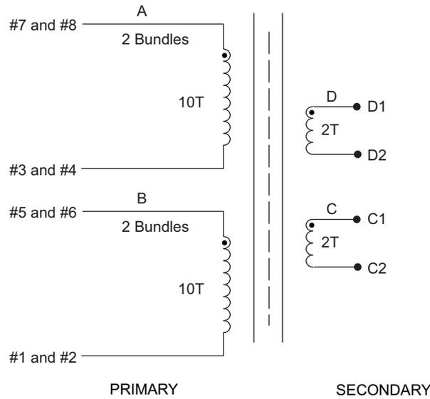
Figure 18. Transformer Schematic
