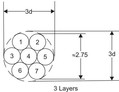
**Figure 17. 7 Conductors**
