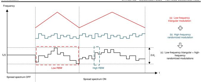
Figure 8-3. Dual Random Spread Spectrum Implementation
