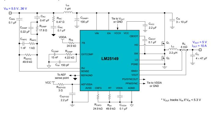
Figure 9-18. Application Circuit 2 With LM25149 Buck Regulator at 440 kHz
