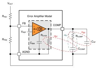
Figure 9-4. Error Amplifier and Compensation Network
