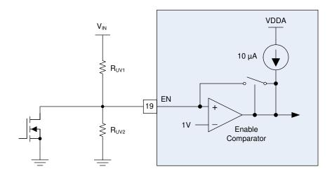
Figure 8-1. Programmable Input Voltage UVLO Turn-On
