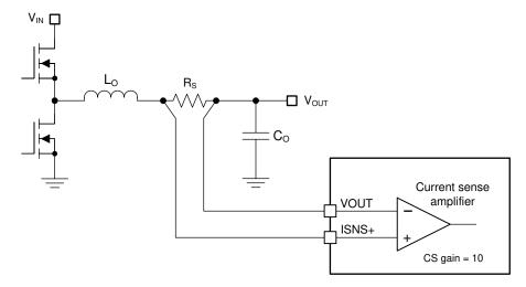
Figure 8-4. Shunt Current Sensing Implementation
