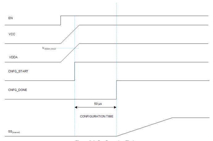
Figure 8-6. Configuration Timing
