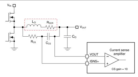
Figure 8-5. Inductor DCR Current Sensing Implementation
