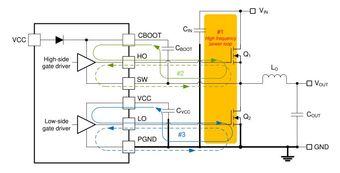
Figure 11-1. DC/DC Regulator Ground System With Power Stage and Gate Drive Circuit Switching Loops
